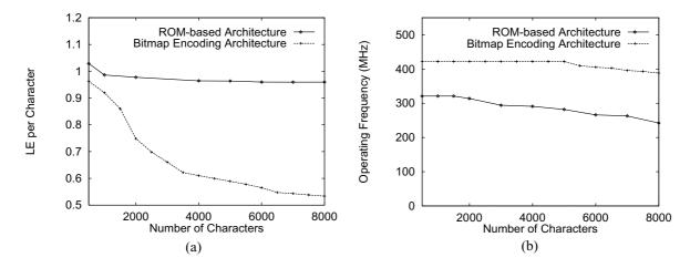
Fig. 10. The performance of the ROM-based and bitmap encoding circuit with q = 1 for various rule sets sizes ranging from 500 characters to 8000 characters (a) LE per character (b) Operating Frequency.
