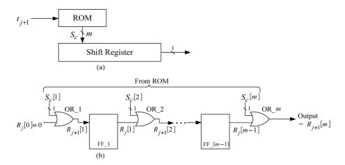
Fig. 3. The basic circuit of each module for exact pattern matching, (a) The block diagram of the circuit, (b) The shift register circuit during clock cycle j + 1.
