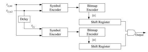
Fig. 9. The structure of a high throughput module circuit processing two characters at a time (q = 2) with the bitmap encoder.
