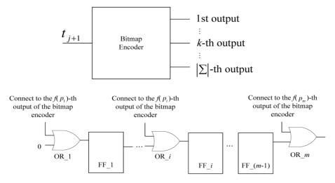
Fig. 4. The shift-or circuit based on a bitmap encoder.
