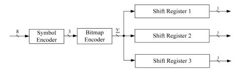
Fig. 8. The sharing of the same symbol encoder and bitmap encoder by three different Snort rules. Each character is also assumed to be an ASCII. All the Snort rules use the same alphabet comprised of 7 symbols.
