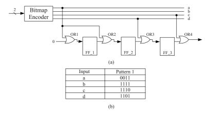
Fig. 5. A simple example of the proposed circuit for the pattern *aadc* and the total symbol *a*, *b*, *c*, *d*, (a)The architecture (b)Table of the pattern.
